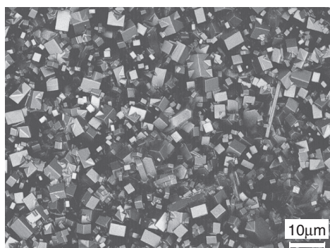
Figure 1. Surface photograph of silicone-rubber-coated silicalite membrane (Membr. No. S-3).
